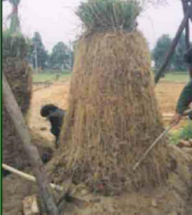
China - excavated root. Average tensile root strength 75 MPa
